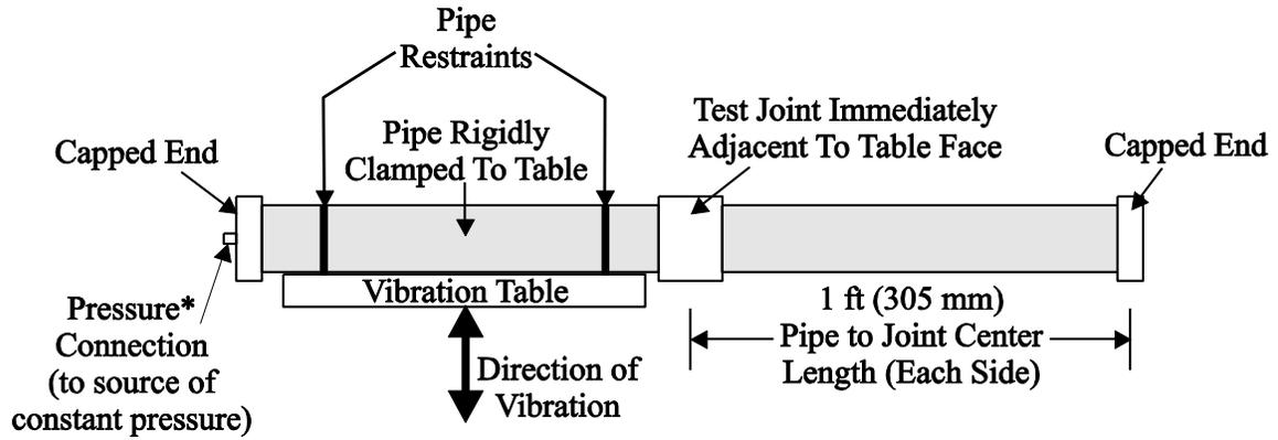
**\*End Caps shall be drilled and tapped to 3/8 or 1/2 inch NPT in order to make use of standard connections. Manufacturer to supply connectors if other than NPT.**
