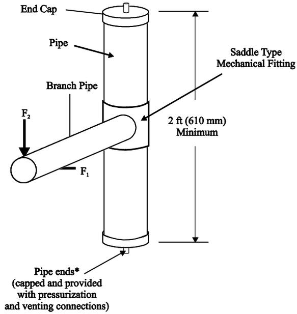
\*End caps shall be drilled and tapped to 3/8 or 1/2 inch NPT in order to make use of standard connectors. Manufacturer to supply connectors if other than NPT.
