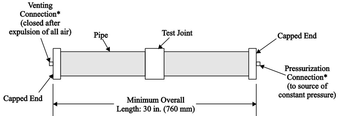
**\*End caps shall be drilled and tapped to 3/8 or 1/2 inch NPT in order to make use of standard connectors. Manufacturer to supply connectors if other than NPT.**
