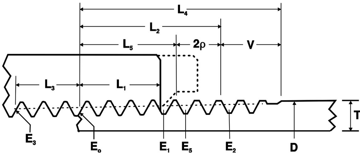
Establish the pitch diameter at the pipe end ( $E_0$ ) for NPS 2 (DN 50) Schedule 40 pipe:
