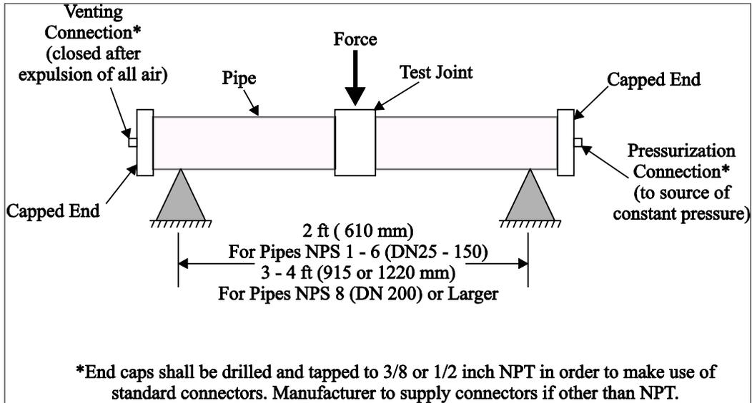
Figure C-3. Rotational Torque Tests
